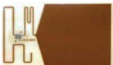
Figure 31 : *Tag* RFID UHF
